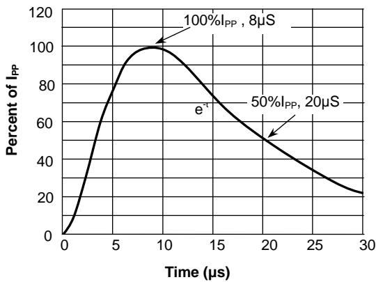
**Fig.4 Pulse Waveform-ESD(IEC61000-4-2)**
